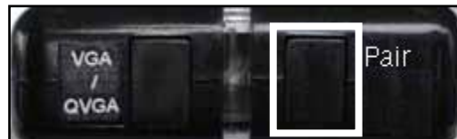
Figure 5.0 Pair button on the Wireless Receiver
